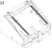
This tool requires little effort to operate and is designed to produce uniform results every time. The Power Assist® Box is controlled by the box handle. These handles come in multiple lengths from 34" to 72", an XTender® Handle that adjusts between 41" and 63" and the 8000TT-PA Wizard™ Compact Finishing Box Handle. The handle is attached to the box by sliding the box onto then handle and tightening the two wing nuts.
