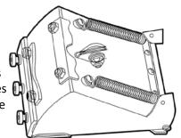
Use the EasyClean® Pump with the box and slot adapter to fill the nail spotter, making sure the joint compound is well mixed and lump free. Normally, no water needs to be added to thin the compound mixture.
